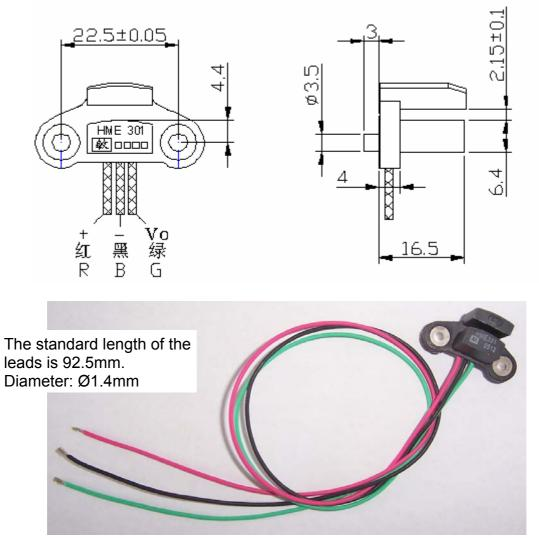
The type and length of the leads can be made according to customer's requirements
